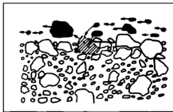
Fig. 10. Schematization of vertical winnowing of fine particles.
