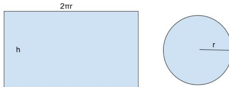
Figure 3.6.9.2: Surface area of the curved side and the area of the bottom
