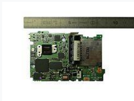
Image sensor (upper left) on the motherboard of a Nikon Coolpix L2 6 MP
