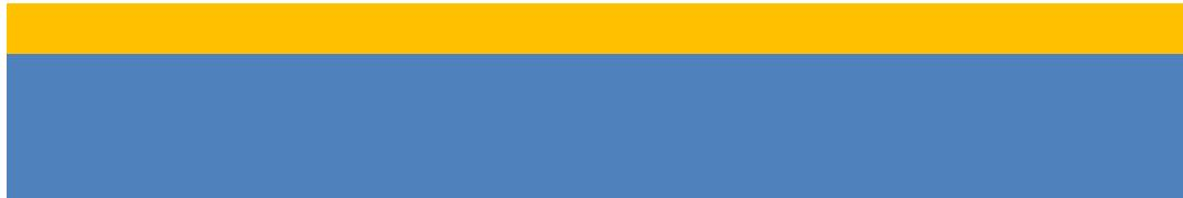
Grow  $\text{SiO}_2$  on top of Si wafer
