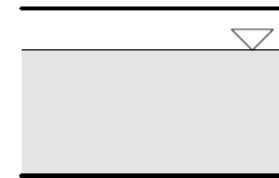
Low oil level in an oil-insulated apparatus
