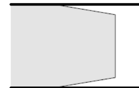
Low oil level in an oil-insulated apparatus
